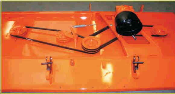
The indirect, flexible V-belt drive of all rotor spindles protects the gearbox and the PTO shaft against shockloads. V-belt tension is easily adjustable. Most belts have an automatic spring loaded belt tensioner.
