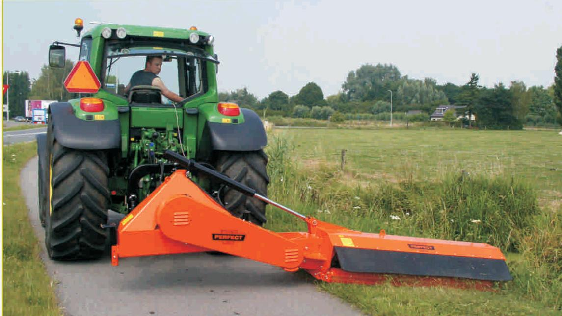
The ZF2 is a very robust professional Articular Offset Flail Mower, designed specifically for the maintenance of roadside verges, embankments, ditch sides etc.
