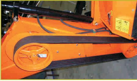
Drive to the flail rotor is transmitted through a 5-fold power belt, which is automatically kept at the right tension. A flexible coupler eliminates peak strokes on the drive system.
