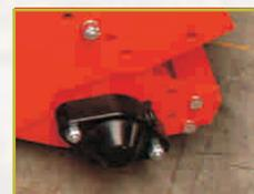
To protect the bearings of the rear roller, the bearings are fitted with unique covers to prevent humidity, dust and mud from entering.
