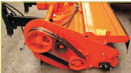
V-belts are kept at the right tension by springloaded automatic belt tensioners. This indirect flexible drive ensures maximum security and requires minimum maintenance.
