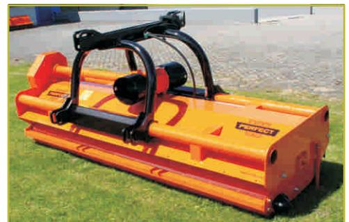
To protect the bearings of the large diameter rear roller, the bearings are fitted with unique covers to prevent humidity, dust and mud from entering.
