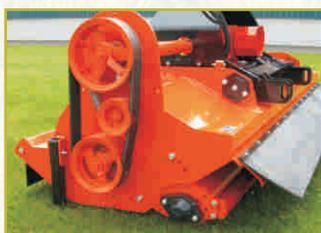
V-belts are kept at the right tension by springloaded automatic belt tensioners. This indirect flexible drive ensures maximum security and requires minimum maintenance.
